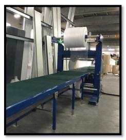
\* Mod. with conveyor belts (optional) automatic top presses (optional) and automatic bubble wrap dispenser (optional).
