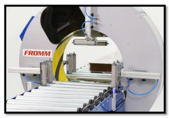
\*Mod. with driven conveyors (optional) and automatic top and lateral presses (optional).
