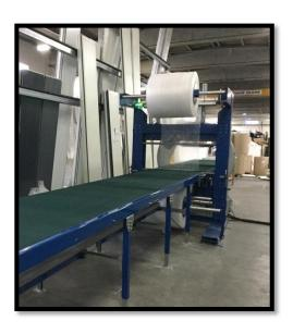
\* Mod. with conveyor belts (optional) automatic top presses (optional) and automatic bubble wrap dispenser (optional)
